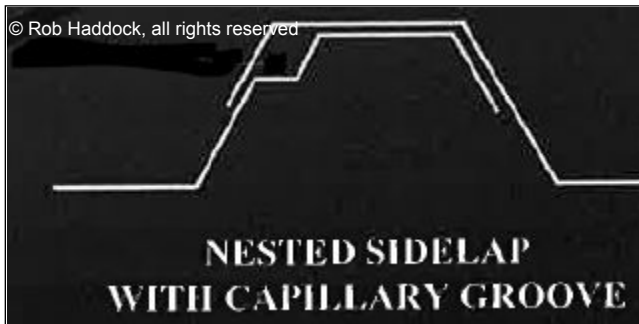
Figure 15-4 Addition of a Capillary Groove to a Nested Seam
