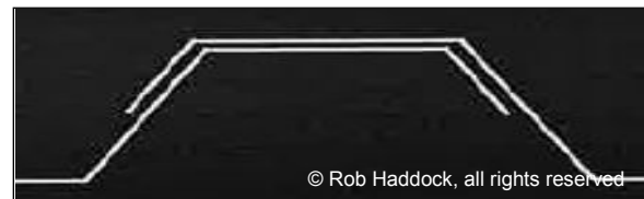
Figure 15-2 The Nested Lap Joint
