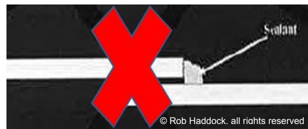
Figure 15-15 Butyl Sealant Should NOT be Externally Applied
