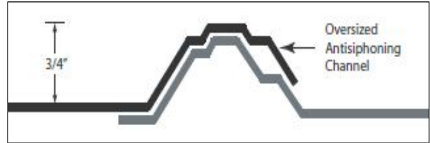
Figure 5-7 Typical Trapezoidal Rib with Overlap Seam
