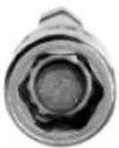
Care should be taken to remove metal chips that accumulate in the magnet socket so that the hex of the screw is embedded completely into the socket.
