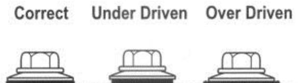
(Note: this image is for general consideration. The fastener manufacturer should be consulted for recommended tightening guidance)
