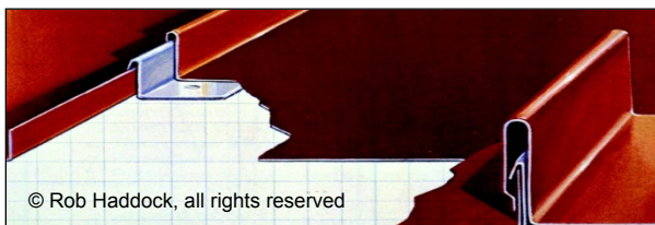
Figure 7-14 Larger Side Ribs Are Used To Conceal Panel Fasteners
