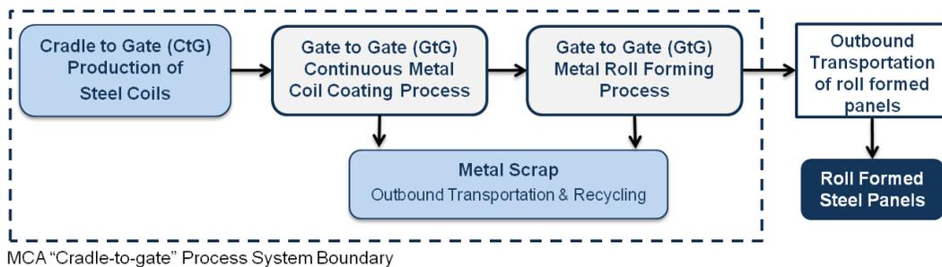
**Figure 8: Cradle-to-Gate System Boundaries of Roll Formed Metal Cladding**
