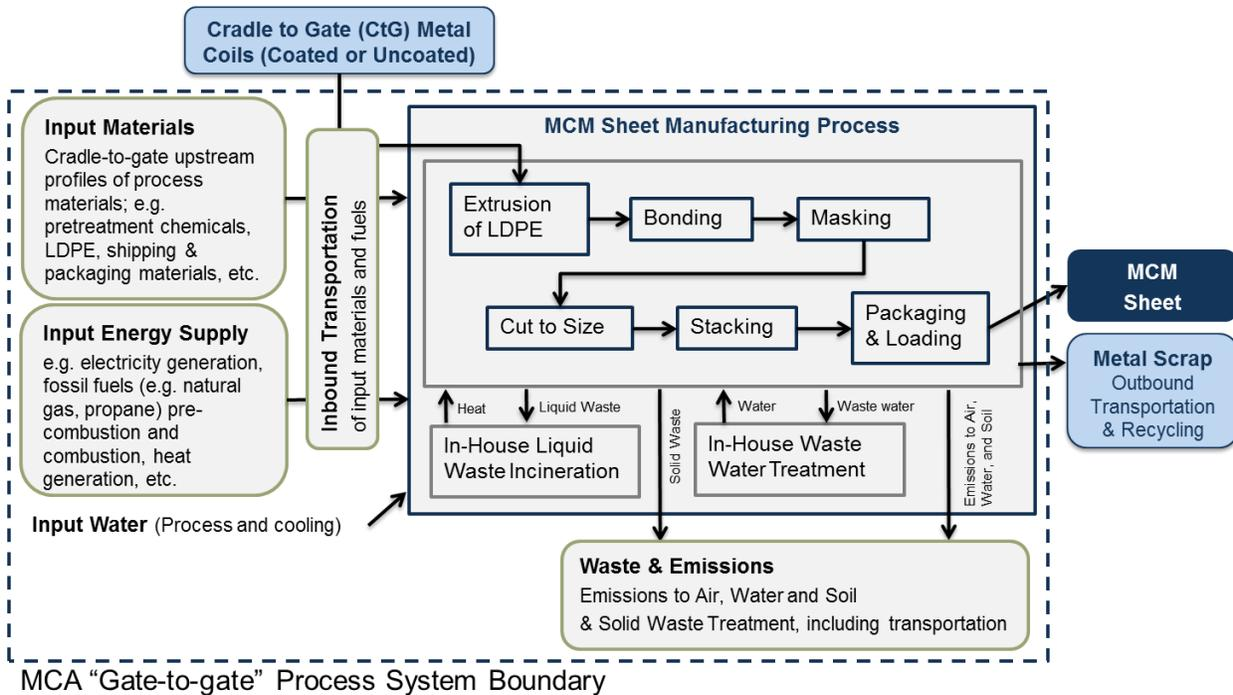
Figure 3: Gate-to-Gate System Boundary of the MCM Sheet Manufacturing Process
