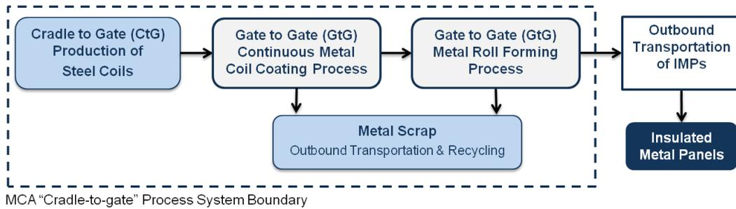
**Figure 6: Cradle-to-Gate System Boundaries of IMP Products**
