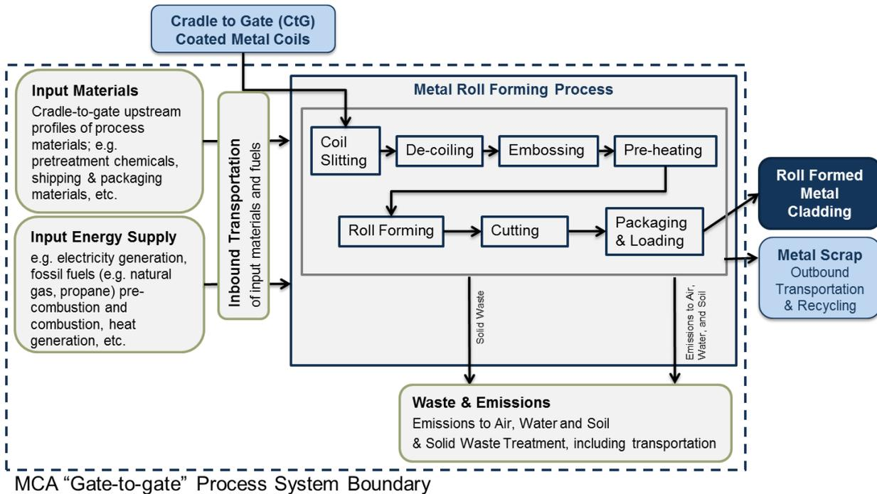
**Figure 5: Gate-to-Gate System Boundary of the Metal Roll Forming Process**
