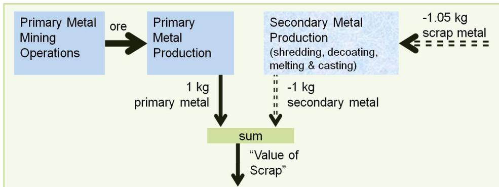
**Figure 9: Value of Scrap as applied in a Life Cycle**
