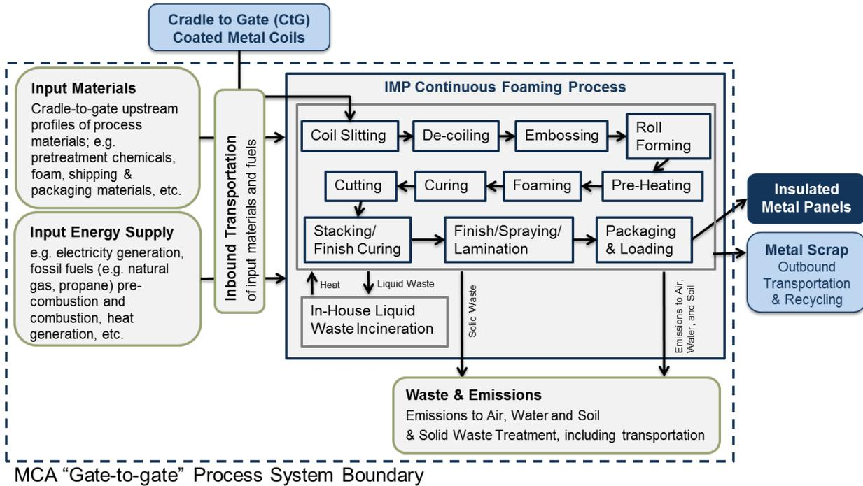
Figure 2: Gate-to-Gate System Boundary of the IMP Continuous Foaming Process
