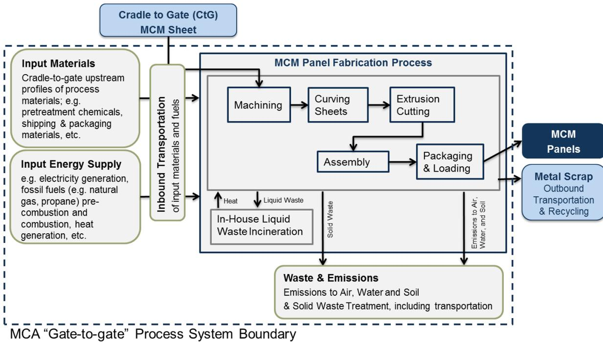
**Figure 4: Gate-to-Gate System Boundary of the MCM Panel Fabrication Process**
