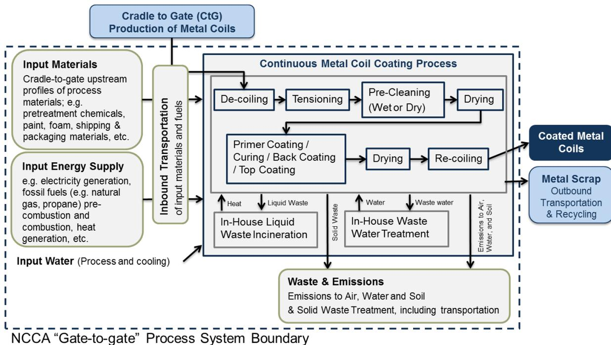
Figure 1: Gate-to-Gate System Boundary of the Continuous Coil Coating Process
