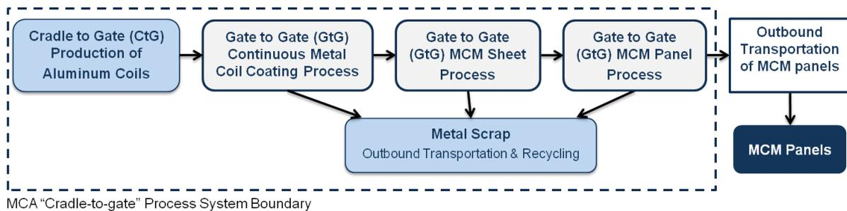
**Figure 7: Cradle-to-Gate System Boundaries of MCM Panel Products**
