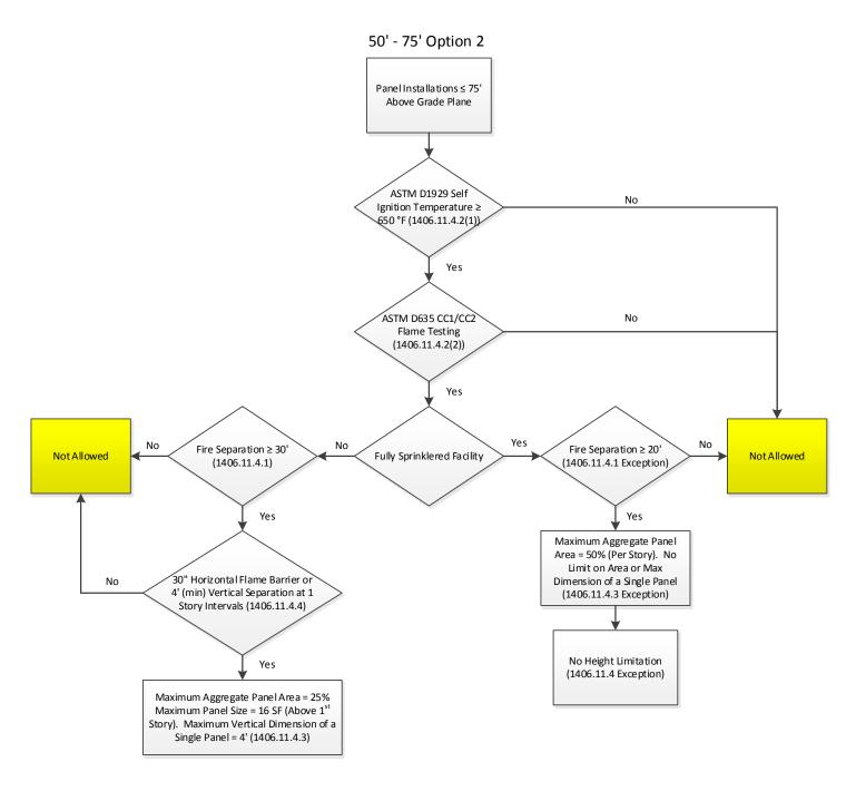
Installations up to 75' above grade plane defined in Section 1406.11.4 (Option 2). Based on the allowable use of light transmitting plastic glazing (Section 2608)
