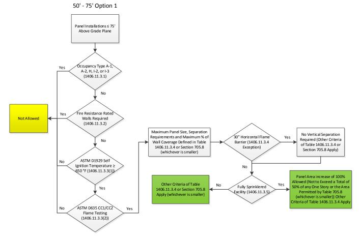
Installations up to 75' above grade plane defined in Section 1406.11.3 (Option 1). Based on the allowable use of light transmitting plastic wall panels (Section 2607)
