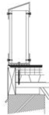
Figure 4-D: “Elevated” low eave wall
