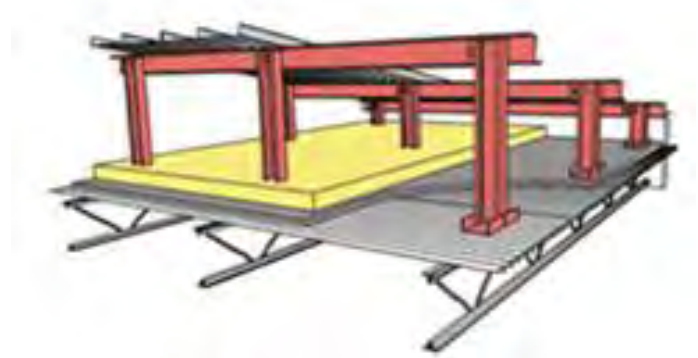
Figure 4-G: Parallel condition bar joist with intermediate base member (Courtesy of McElroy Metals)
