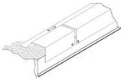
Figure 4-B: “Fixed” elevation Low-eave member
