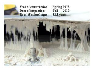
Any sealant used in latent metal construction details should be intended for long life as it is not easily repaired or replaced without potential damage to panels or other parts. Such details should accommodate expected movement through the design of the joint itself, not purely by sealant deformation.
