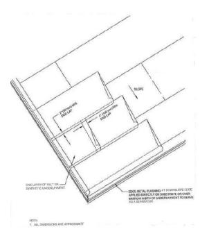
Figure 10-16 Underlayment over Rigid Insulation
