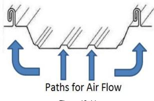
Figure 10-11 Ventilation Provided by Panel Profile
