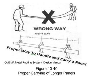
An installer **does** have control over these installation and handling issues. Instructions to additional labor, erection, and roofing crew members regarding proper handling, spacing, and fastening should be presented based on the manufacturers' material.
