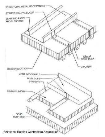
Figure 10-14 Insulation over Solid Deck with Purlins
