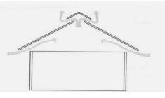
Figure 10-8 Typical Air Flow for Roof Ventilation
