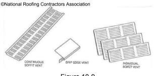
Figure 10-9 Eave and Soffit Vent Examples
