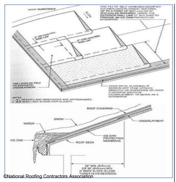
Figure 10-25 Typical Ice Dam Membrane Installation
