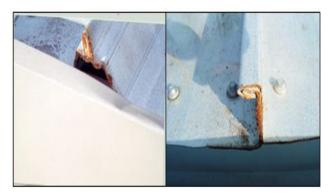
Figure 10-44 Burrs and Sharp Edges Snag Debris
