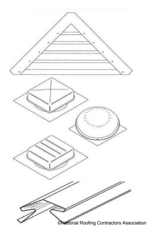
Figure 10-10 Examples of Common Ridge and Gable Vent Styles
