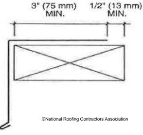
Figure 10-55 Nailer Details for Drip Edge Material
