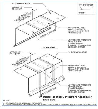
Figure 10-52 Drip Edge with Overlapping Joint Plate
