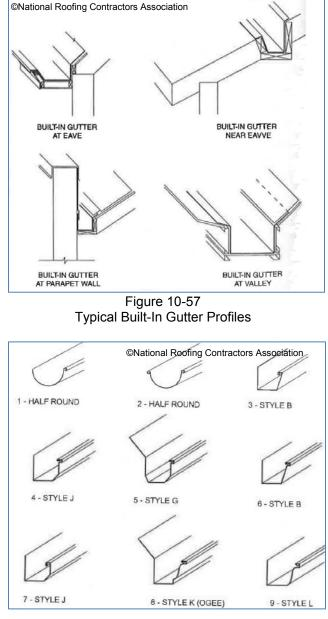
Figure 10-58 Typical Hanging Gutter Profiles
