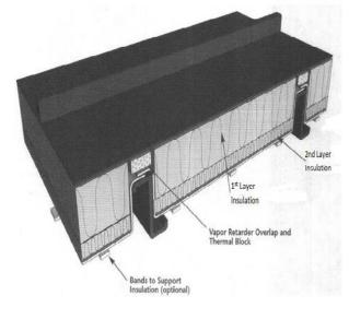
Figure 10-20 Roll Insulation Between Purlins Using Thermal Blocks
