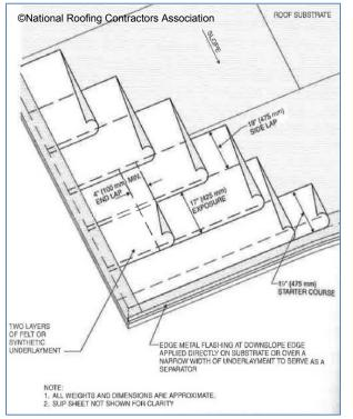
Figure 10-28 Double-Layer Underlayment Installation
