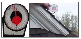
Figure 10-85 Slope Measurement Tool
