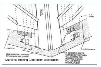
Figure 10-70 Stripping of Clip-Installed Valley Trim
