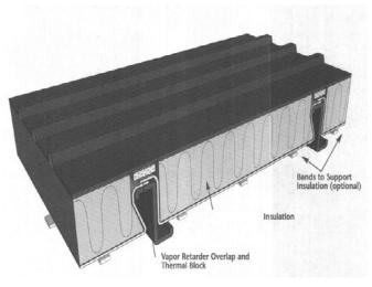
Figure 10-18 Roll Insulation Between Purlins
