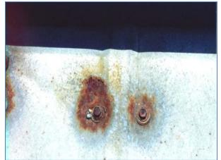
Figure 10-48 Incorrect Fastener Material
