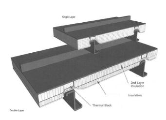
Figure 10-19 Roll Insulation over Purlins Using Thermal Blocks
