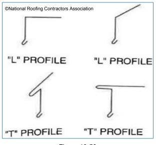
Figure 10-50 L and T style Drip Edge Profiles
