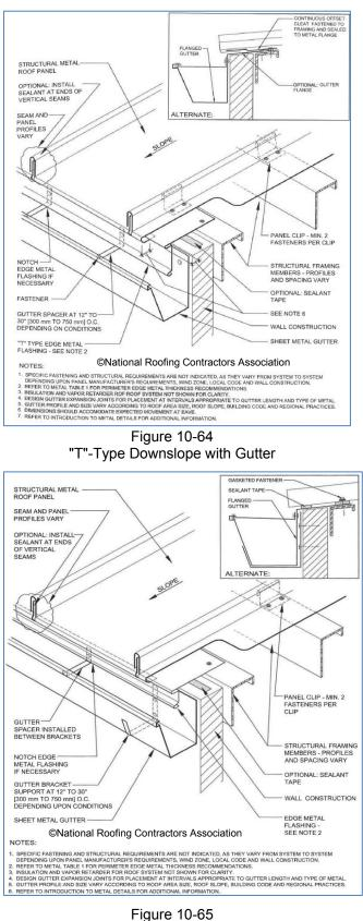
"T"-Type Downslope with Gutter and Brackets
