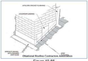
Figure 10-66 Apron Flashing Around a Chimney
