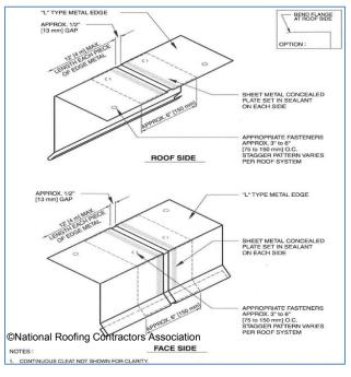
Figure 10-53 Drip Edge with Concealed Joint Plate
