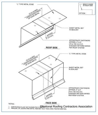
Figure 10-51 Overlapping of Drip Edge Material
