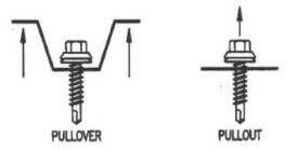
©MBMA Metal Roofing Systems Design Manual Figure 10-4 Fastener Pullover and Pullout Factors
