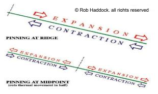
Figure 10-35 Pinning at Midpoint Cuts Thermal Movement in Half
