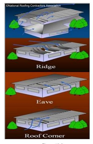
Figure 10-3 Potential Areas of Roof Wind Damage
