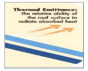
Figure 10-7 Thermal Emittance, Radiating Absorbed Heat
