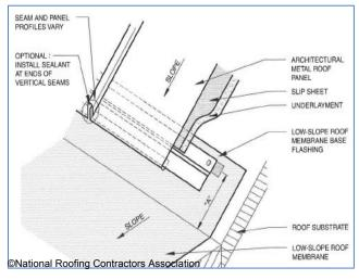
Figure 10-81 Transition from Metal Roof to Membrane Roof
