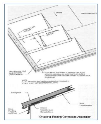
Figure 10-27 Typical Single Layer Underlayment Installation
