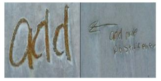
Figure 10-45 Corrosion Caused by Graphite Pencil
