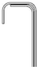
The unseamed panels must be installed and nested together properly before seaming can begin.
