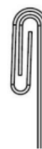
This seam type is commonly referred to as a 180° seam by the additional 90° of travel that the material moved from the 90° profile.
