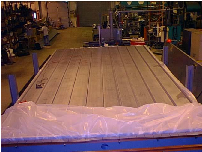
Fig. 1 ASTM E1592 Static Load Roof Test Setup
