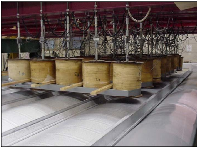
Fig. 3 Magnetic Uplift Load Test
