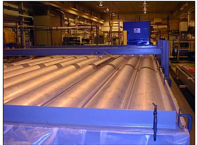
Fig. 2 Deformed Roof Panels during ASTM E1592 Test
