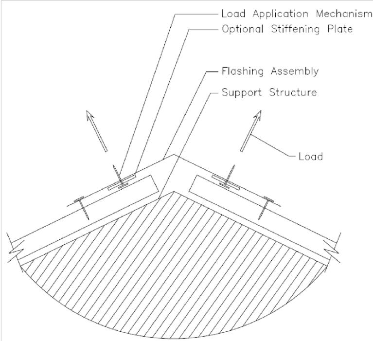
Figure 3 – Two Load Test Apparatus
