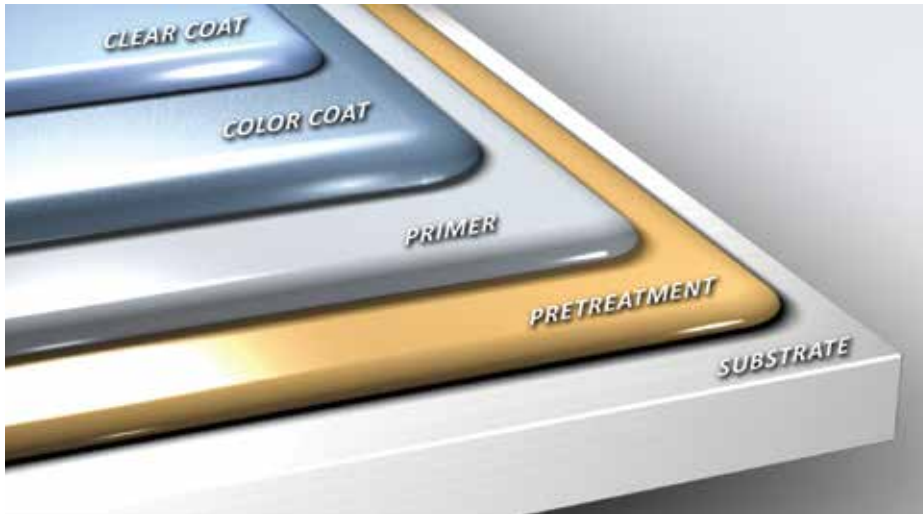
This illustration shows the layers of an MCM panel.
