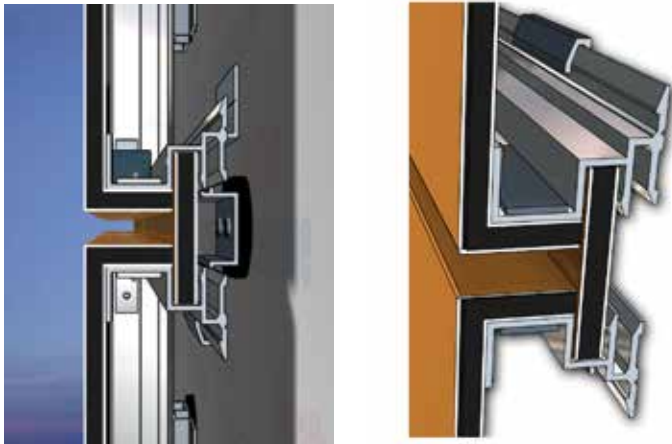
This illustration shows the back skin and a portion of the MCM core.
